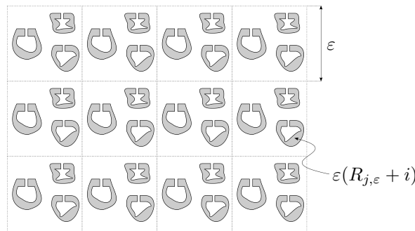
Fig. 1.2: The domain \Omega_\varepsilon , here m = 3 . The dotted lattice separates different period cells.
